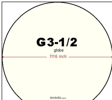
usual shape of G3-1/2 glass envelopes (not to scale)
